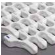
S.201 Open radius belt with a very low collapse factor. Can run in S- and J-curves for spiral coolers/freezers as well as normal radius applications.
