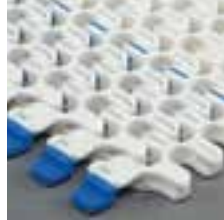
S.101TAB Open radius belt with a very low collapse factor. Can run in S- and J-curves for normal radius applications.
